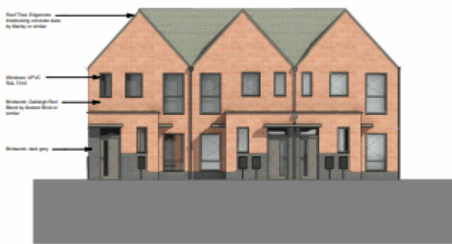
Front (North) Elevation 1 : 100
